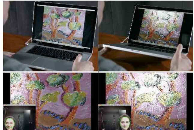
Figure 2. Image sequence showing a model of an oil painting being displayed on the tangiBook laptop. Custom software allows the orientation of the laptop screen and the position of the screen observer to be tracked in real-time. Tilting the laptop or moving in front of the screen produces realistic changes in surface lighting and material appearance.
