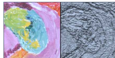
Figure 3. The left image shows a section of the color map of a painting and the right image shows the associated height map.
