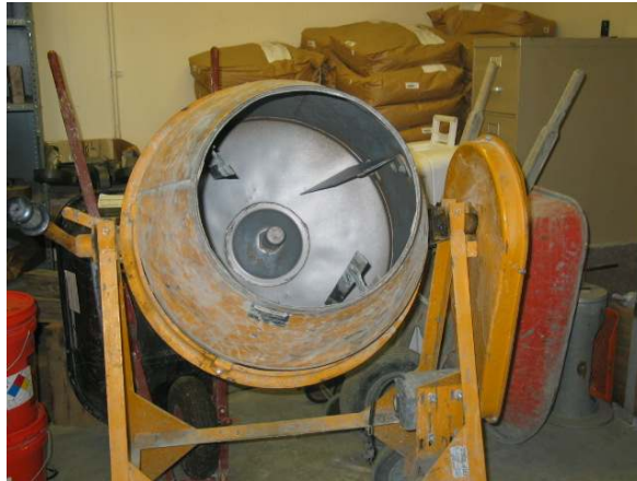
Figure 2-1. Three cubic-foot concrete mixer used to prepare samples for grout formulation development.
