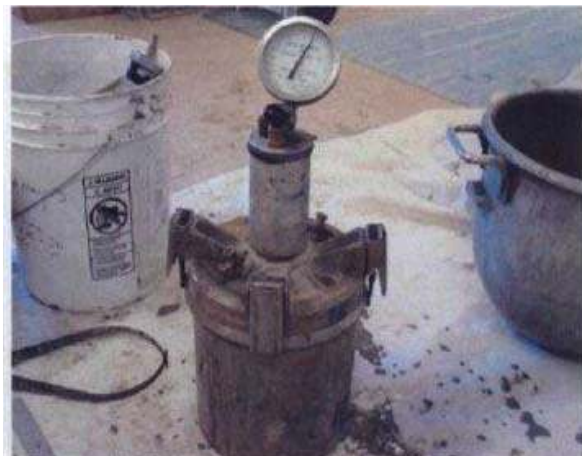
Figure 2-3. Air content test apparatus and including unit weight bucket.
