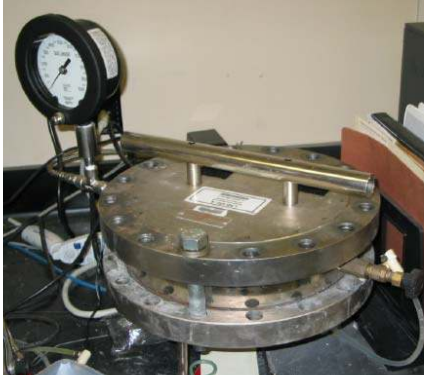
Figure 2-6. Pressure plate test configuration for moisture retention characterization.
