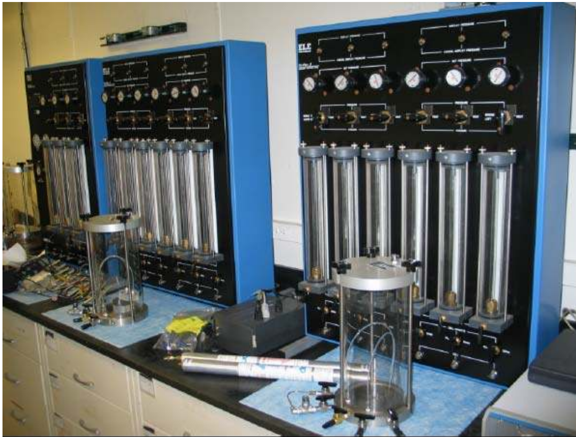
Figure 2-5. Hydraulic conductivity test apparatus and sample cells.
