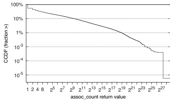
Figure 4: assoc_count frequency in our production environment. 1% of returned counts were \geq 512K .
