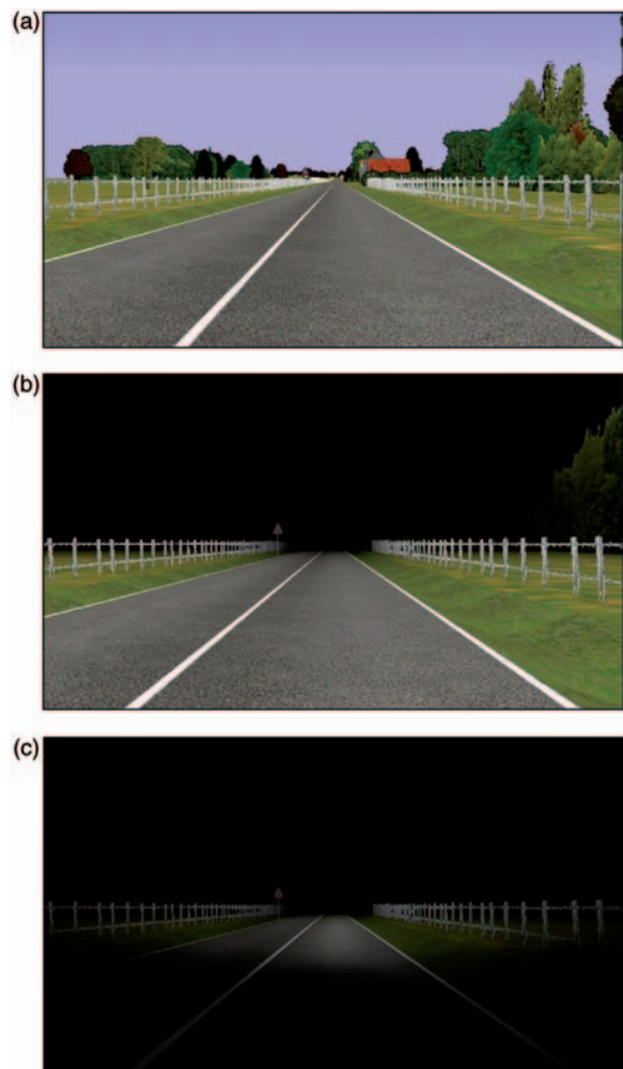
Figure 1 Three-step special effect to simulate headlight illumination conditions: (a) daytime scene, (b) with black fog and (c) with headlamp beam pattern texture. (Available in colour in electronic version of paper.)
