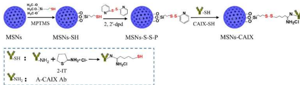
Scheme 2. Synthetic route of CAIX targeted mesoporous silica nanoparticles “MSNs-CAIX”.
