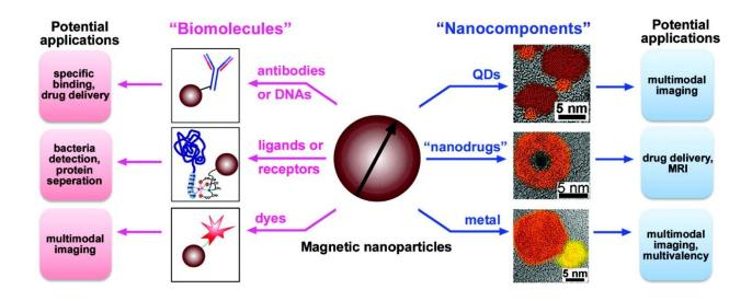
FIGURE 3 TWO STRATEGIES TO FABRICATE MULTIFUNCTIONAL MAGNETIC NANOPARTICLES AND THEIR POTENTIAL APPLICATIONS
