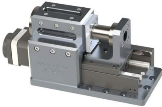
Figure 11. Adjustable length gas cell developed by SourceLAB. Courtesy of F. Sylla.
