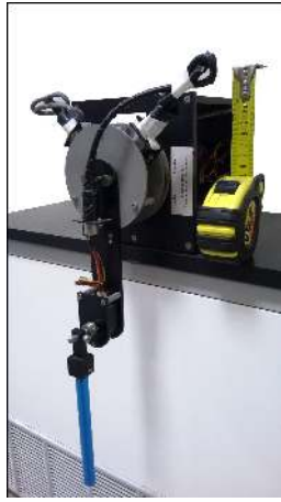
Fig. 2. The Pendubot available in our laboratory and used in our planning experiments.
