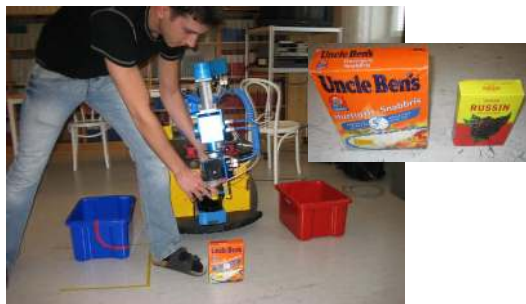
Fig. 5. The user drags the robot arm to show it how to grasp the object, and move the object to the bin.
