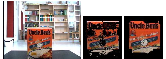
Fig. 4. Left: The original image. Center: The result after image differencing. Right: The result after morphological operations
