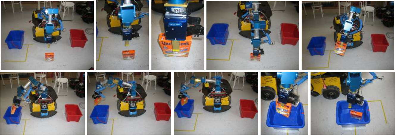
Fig. 6. The robot executing the task. The rice package has been recognized and moved to the left bin as demonstrated by the user.
