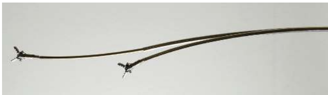
Fig. 2. Two overlaid time frames of a concentric tube robot. As the inner tube is extended past the outer tube, the inner tube interacts with the outer tube’s curvature, causing the entire robot’s shape to change. This illustrates that the tubes cannot necessarily be treated as kinematically independent during the design and control of these robots.
