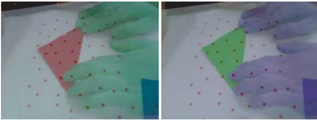
Figure 16: Synthesis results of RGB swapping: (Left) usual image, (Middle) image obtained by swapping RGB with GBR and (Right) image obtained by swapping RGB with BRG
