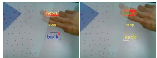
Figure 4: Detection of the AR-button: (Left) is not enough, and (Right) is enough
