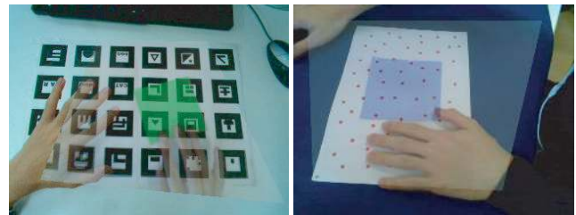
Figure 7: Fitting the marker and the system: (Left) in the case of using the ARToolKit marker and (Right) in the case of using a point marker
