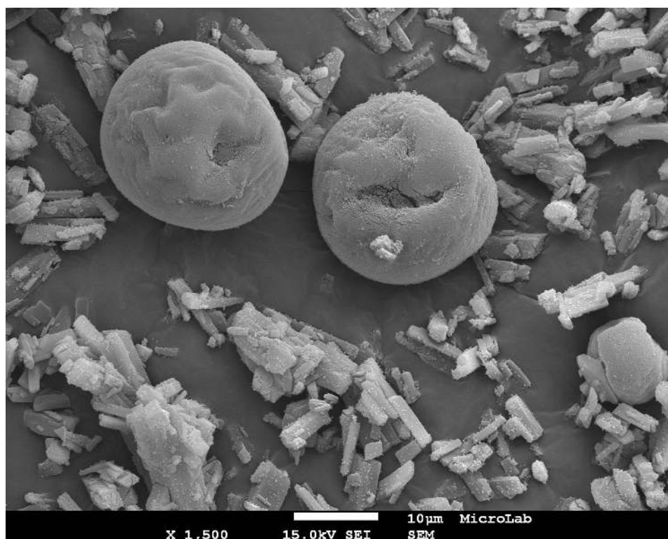
Figure B.1 SEM micrograph correspondent to the physical mixture (blend drug:polymer in the same proportion used to produce the formulations, 60:40 % wt.) at a magnification of 1 500x.
