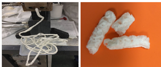
Fig. 5. Representative picture showing the foaming of extrudates when plasticizers (xylitol, sorbitol, mannitol, and erythritol) were used at lower concentration (10% w/w)
