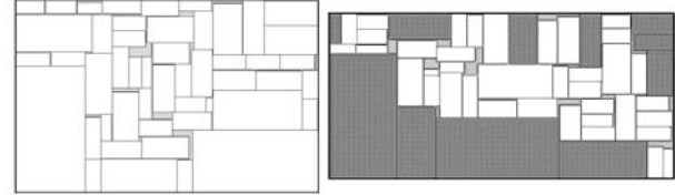
Figure 6: Resulting placements of ami49 (1) left: area optimization (area = 36.398mm^2 ); (2) right: placement with boundary modules being heavily shaded ( (|T|, |B|, |L|, |R|) = (3, 3, 2, 3) , area = 36.765mm^2 ). Note that the lightly shaded regions denote dead spaces.
