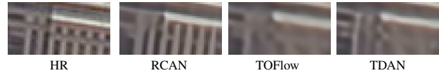
Figure 8. A failure case of the TDAN. The very deep SISR network: RCAN can accurately recover the structures of the shown image region in the city video frame, but TOFlow and TDAN fail.
