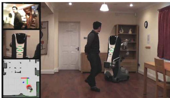
Fig. 1. Interior of the robot house “living room” with the Care-O-Bot3 robot. The images on the left side of the picture show the view from the robot camera, the robot itself, and the real-time mapping visualization showing person and robot location.
