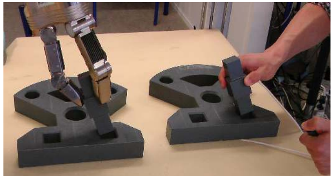
Fig. 6. Control of the robot in teleoperation mode. The robot performs a one-to-one copy of the human demonstrated path.
