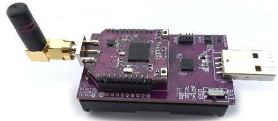
Fig. 2. The OpenMote platform with the OpenUSB carrier board. The OpenUSB contains various sensors (temperature, relative humidity, light, 3-axis acceleration) and allows a user to reprogram it over USB.
