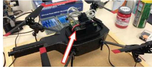
Figure 6. Custom AR.Drone with auxiliary embedded board.
