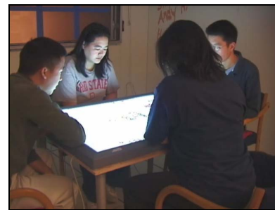
Figure 1. A four-person group uses TeamSearch at a DiamondTouch table to find photos from a metadata-tagged repository.
