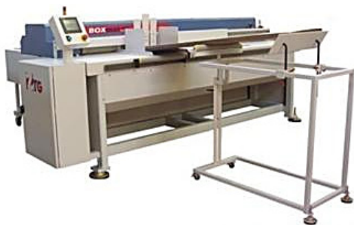
Fig. 9. Boxmat 2400 - automatic slotted-type box making machine [20]
