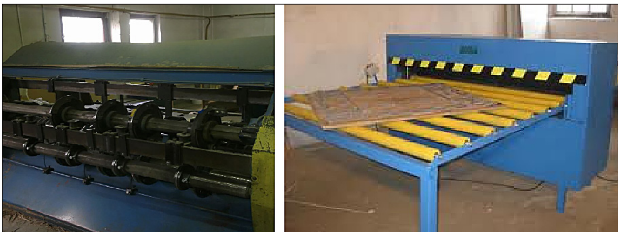
Fig. 3. Technical equipment: a) slotter, b) roller die cutter
