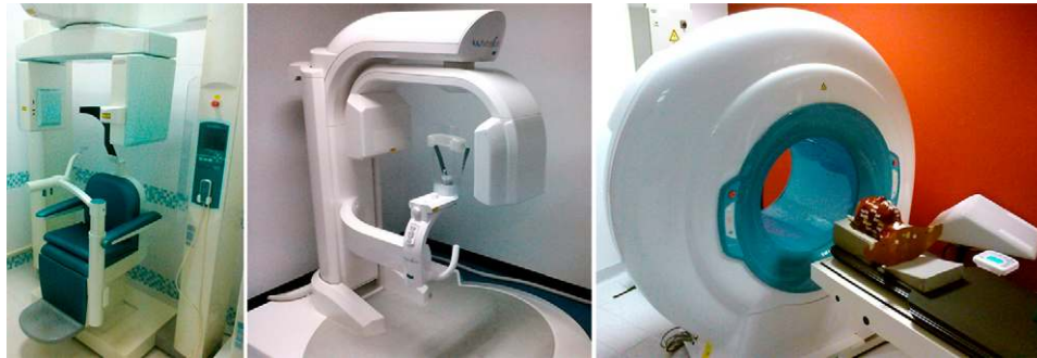
Figure 4 Different types of CBCT gantries. Left: seated patient position (3D Accuitomo ® 170; J. Morita, Kyoto, Japan). Middle: standing patient position (WhiteFox ® ; Acteon Group, Mérignac, France). Right: supine patient position (NewTom ® 5G, QR srl, Verona, Italy).
