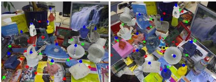
Fig. 1. 15 different texture-less 3D objects are simultaneously detected with our approach under different poses on heavy cluttered background with partial occlusion. Each detected object is augmented with its 3D model. We also show the corresponding coordinate systems. See supplemental video.
