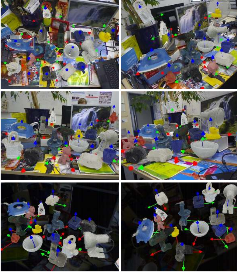
Fig. 4. 15 different texture-less 3D objects are simultaneously detected under different poses on heavy cluttered background with partial occlusion and illumination changes. Each detected object is augmented with its 3D model. We also show the corresponding coordinate systems. See also the supplemental video.
