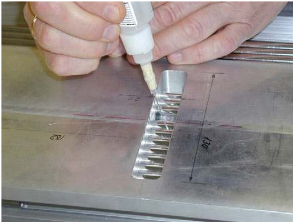
Fig. 26. Gluing of straw tubes to multi-layers.
