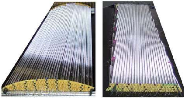
Fig. 24. Photograph of an axial straw layer module for the outer cylindrical shape and module with two double layers with opposite skew angle.
