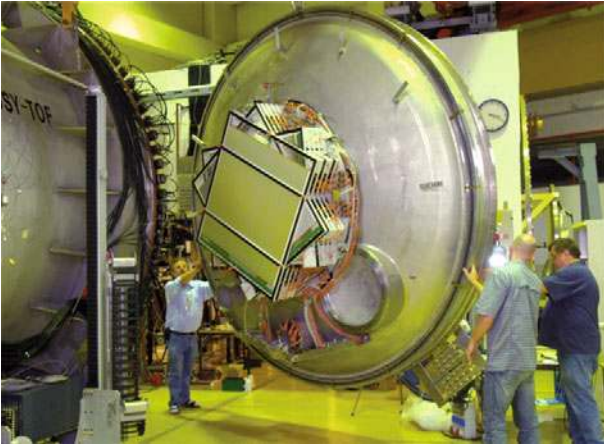
Fig. 66. Mounting of the COSY-STT in the time-of-flight barrel of the COSY-TOF spectrometer.
