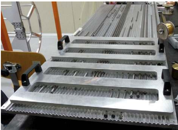
Fig. 182. v-shaped reference plate for multi-layer assembly.
