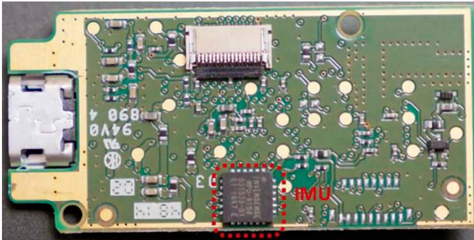
Figure 37: Bottom side of the Myo armband control board: the MPU-9150 IMU is highlighted in red.
