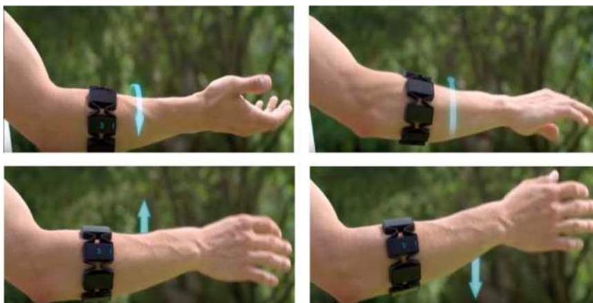
Figure 1: By analyzing electrical activities of forearm muscles, the MYO armband detects hand movements in each direction (Myo Armband web site). Copyright © Thalmic Labs Inc. 2013–2016.
