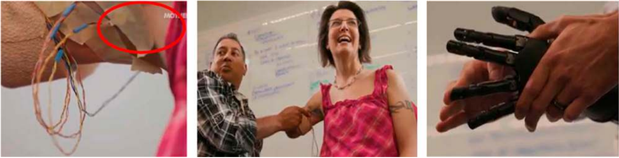
Figure 15: The contact sensors provide feedback signals to the patient that “feels” the touched objects. Copyright © Vice Media Inc. 2016.
