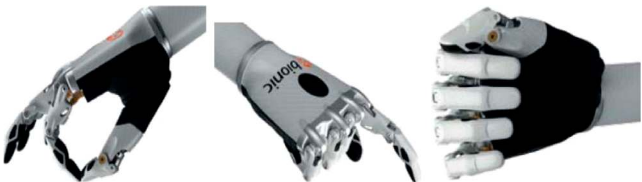
Figure 20: The advanced bionic prosthesis produced by Ottobock allows to independently move each finger in a very precise way. Copyright by Ottobock © 2018.
