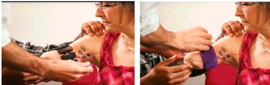
Figure 10: Myo armband worn by the patient; the purple band serves to better tighten the armband around the arm. Copyright © Vice Media Inc. 2016.
