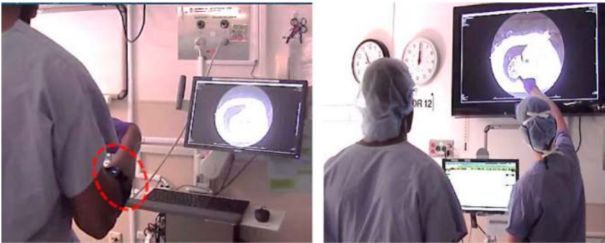
Figure 8: Myo armband used in a surgery room for controlling a camera to visualize the examined body part, without having to physically touch a controller or medical instrument and thus improving user safety and reducing infections risk.
