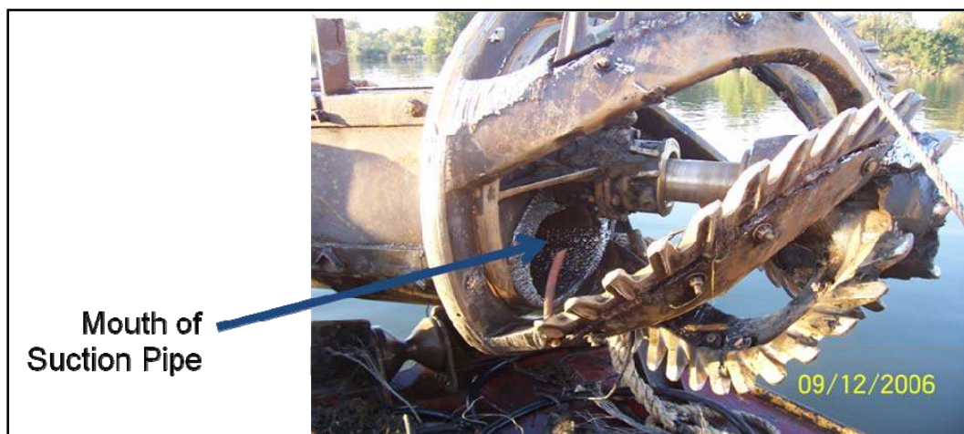
Figure 15. Mouth of suction pipe and conventional basket cutterhead.
