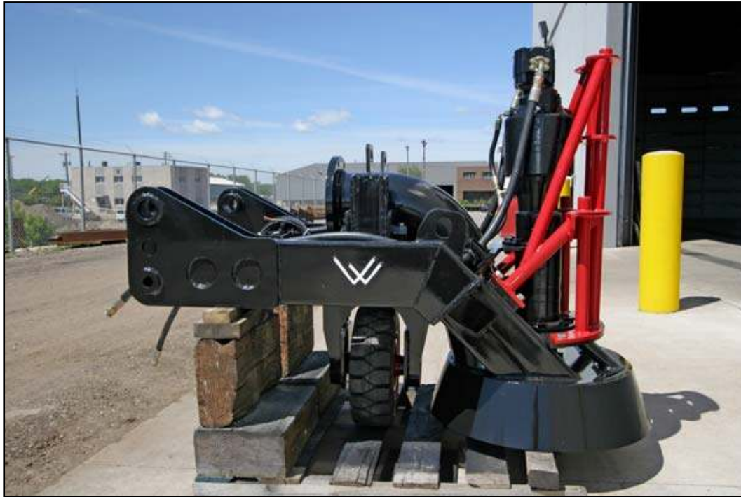
Figure 14. Vic Vac® hydraulic dredgehead for residuals.
