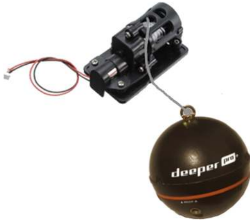
Figure 2. Deeper sonar is connected to a UAV with a wire winch.
