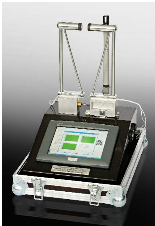
Fig. 3. Calibration system with krypton hygrometer, stepping motor, HMP45A temperature-humidity sensor and touchpanel PC, the switch, fuses and connector for hygrometer at the left side and USB as well as network connector at the right side (photograph: B. Mast)
