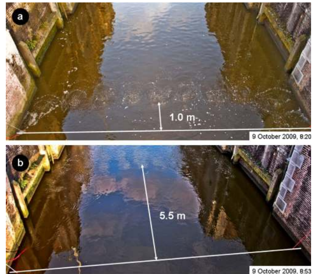
Fig. 7. The bubble envelope during low ( 3.3\text{ m}^3\text{ s}^{-1} ) and high ( 16\text{ m}^3\text{ s}^{-1} ) discharge, respectively.
