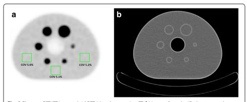
**Fig. 2** Phantom PET/CT images. Axial PET (**a**) and attenuation CT (**b**) images from the IQ phantom on the scanner bed. The phantom spheres and background were filled with FDG activity (ratio 10:1), and the scan duration was 10 min. The *squares* illustrate three ROIs in one axial plane that are used to determine the COV
