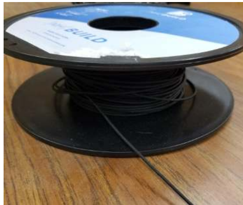
Figure 13. 3-D printing filament made from waste composite.
