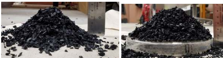
Figure 6. Angle of repose analysis a) pile method and b) petri dish method.
