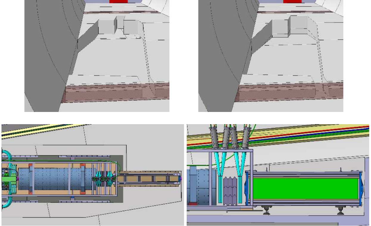
FIG. 4. Top left: The original plans for the FASER trench. Top right: The current shape of the FASER trench. Civil engineering considerations have required the drainage pipe to be redirected, and as a consequence, the front of the trench has been widened and deepened, providing more room for FASER \nu . The trench width around the FASER spectrometer is unchanged. Bottom: Top and side views of the front of the trench. The box on the right indicates the location of FASER \nu , which contains emulsion and tungsten layers and occupies a volume of 30 \text{ cm} \times 30 \text{ cm} \times 1.35 \text{ m} .
