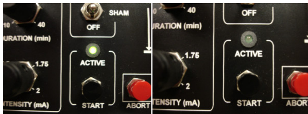
Figure 8. Delivery of active (left) and sham (right) mode by conventional tDCS device. From DaSilva, et al. 19 .
