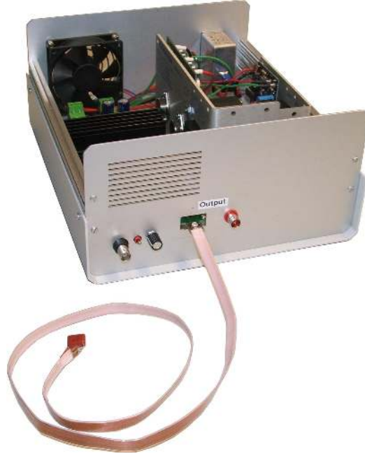
Figure 3. Amplifier enclosure with connected cable and 100 nF capacitive load
