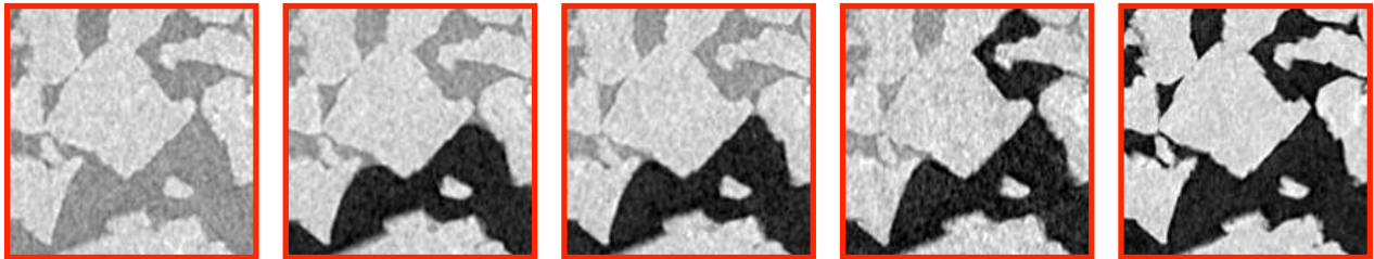
Figure 2: Snapshots of air displacing a NaI-doped water from the pore space of a Bentheimer sandstone sample. Images are 210 \times 210 voxels, taken from 2000^3 datasets. Dynamic tomography has enabled images of this type of fluid displacement to be acquired an order of magnitude faster than with static imaging.
