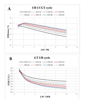
**Figure 9.** (**A**) Effects of the compression ratio with changing LPC in the I/R CCGT cycle. (**B**) Effects of the compression ratio with changing LPC in the I/R GT cycle.
