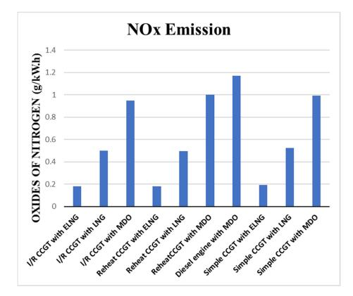
Figure 14. NOx emissions from all propulsion systems.
