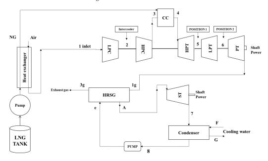
**Figure 4.** ELNG cycle layout. LNG: liquefied natural gas; HPC: high-pressure compressor; LPC: low-pressure compressor; CC: combustion chamber; S.T.: steam turbine; 1: outlet air mass flow temperature from heat exchanger to low-pressure compressor; NG: the outlet natural gas mass flow from heat exchanger to combustion chamber.
