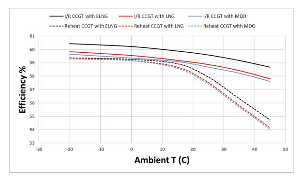
Figure 11. Effects of the ambient temperature on the overall thermal efficiency.
