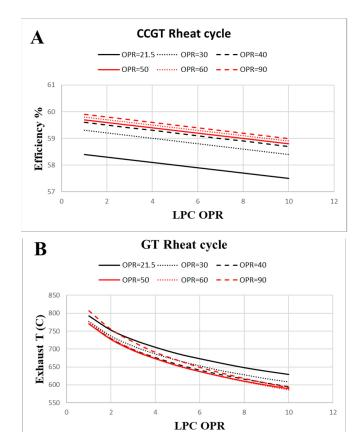
**Figure 8.** (**A**) Effects of the compression ratio with changing LPCs in the reheat CCGT cycle. (**B**) Effects of the compression ratio with changing LPCs in the reheat GT cycle.
