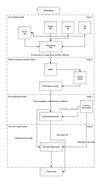
**Figure 1.** Flowchart of the methodology employed in this study. NOx: Nitrogen oxide; CO<sub>2</sub>: carbon dioxide; CCGT: combined-cycle gas turbine (with steam); I/R: intercooler–reheat cycle; HRSG: heat recovery steam generator; ELNG: enhanced liquefied natural gas.
