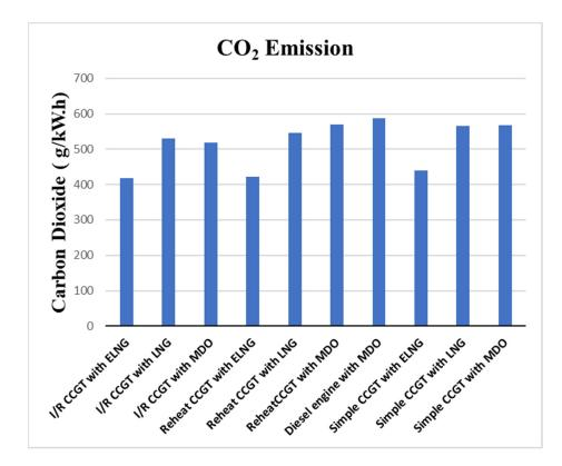
Figure 15. CO<sub>2</sub> emissions from all propulsion systems.
