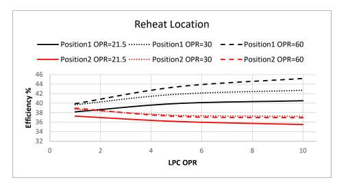
Figure 7. Effects of the compression ratio with different LPCs in the reheat cycle.
