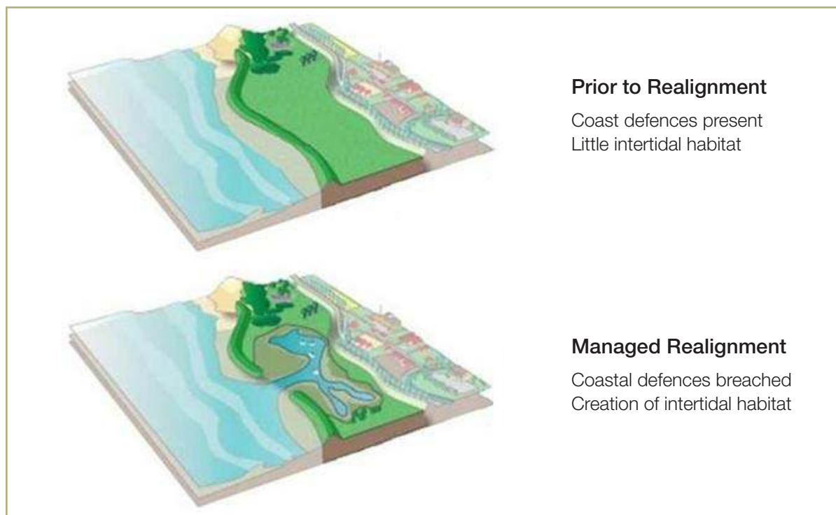
Figure 4.28: The process of managed realignment
