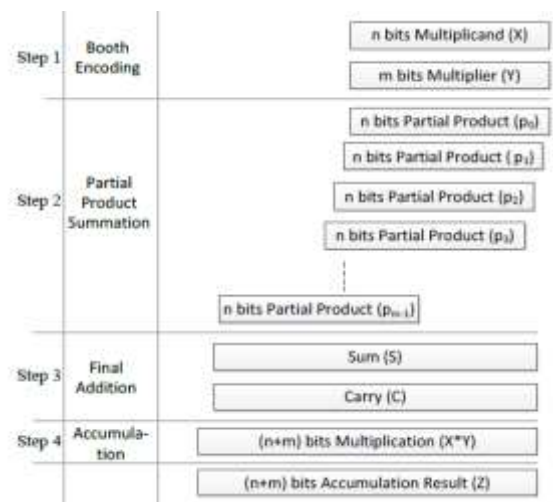
Figure 1: Basic arithmetic steps for multiplication and Accumulation
