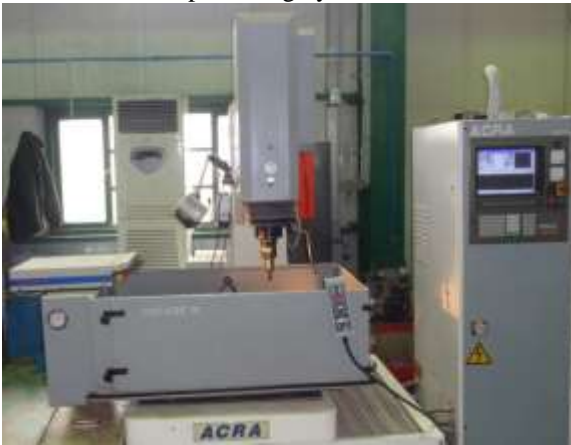
Figure (2): ACRA type CNC-EB EDM machine manufactured by FREJOTH INTERNATIONAL LTD. /TAIWAN
