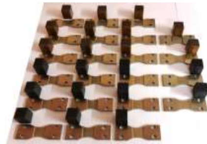
Figure (3): The specimens and the used copper and graphite electrodes for the first and second group of experiments after EDM machining
