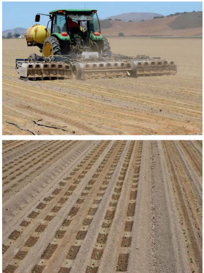
Figure 4. Lettuce thinning at Salinas, CA with the BlueRiver Lettuce Bot (top) and a close-up of the newly thinned lettuce showing the sprayed zones where lettuce will be removed and unsprayed zones where “saved” lettuce plants will be grown to maturity (bottom). (Color for this figure is available in the online version of this article.)
