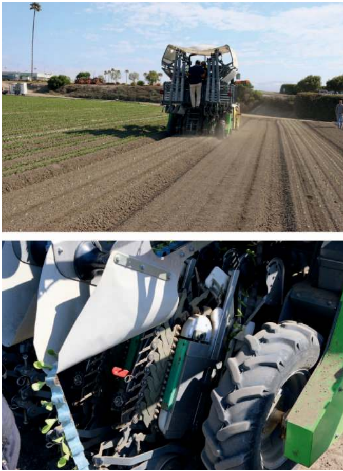
Figure 5. The Plant Tape machine transplanting lettuce with six plant lines per 2-m-wide bed (top) at Spreckles, CA. Shown on the bottom is a close up of one plant tape feeding into the transplant mechanism. (Color for this figure is available in the online version of this article.)
