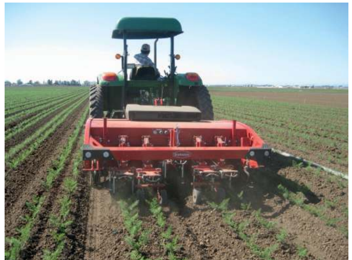
Figure 3. Steketee IC, equipped with reciprocating knives operating in a fennel ( Foeniculum vulgare Mill.) planting near Castroville, CA. (Color for this figure is available in the online version of this article.)
