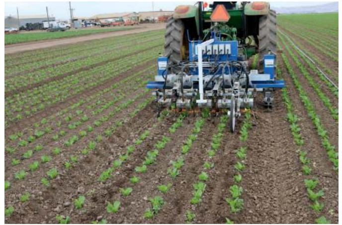
Figure 2. Robovator intrarow cultivator equipped with reciprocating knives, weeding lettuce on a 2-m-wide bed near Santa Maria, CA. (Color for this figure is available in the online version of this article.)
