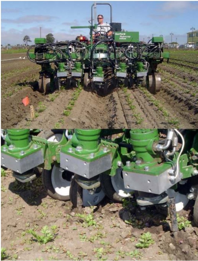
Figure 1. Robocrop intrarow cultivator used on two celery [ Apium graveolens L. var. dulce (Mill.) DC.] beds at Salinas, CA (top). The bottom photo is a close up of the intrarow cultivation. (Color for this figure is available in the online version of this article.)
