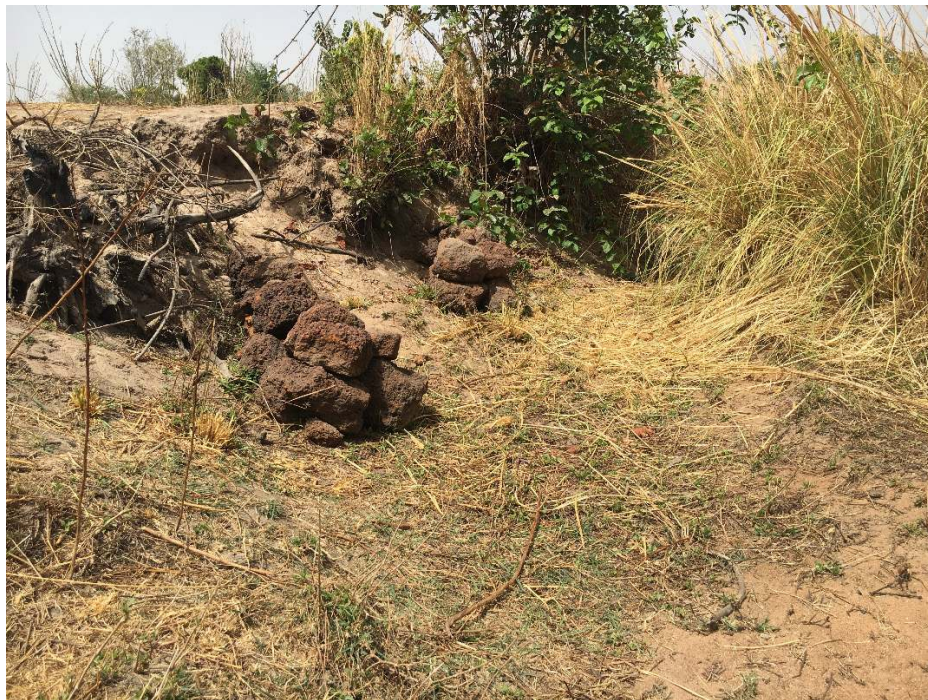
Figure 16. Photo of 2 groynes built and placed at the end of the test site. (photo by author).
