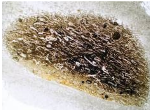
Figure 6: Husk and grog material, Ancient Subjumba, Sample 5, Central Region, PPL magnification 10x
