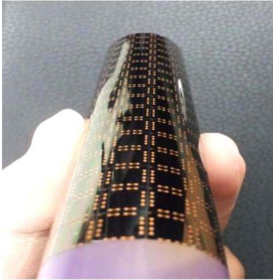
Fig. 11. Picture of flexible semiconductor memory developed by Hanamicon Co.
