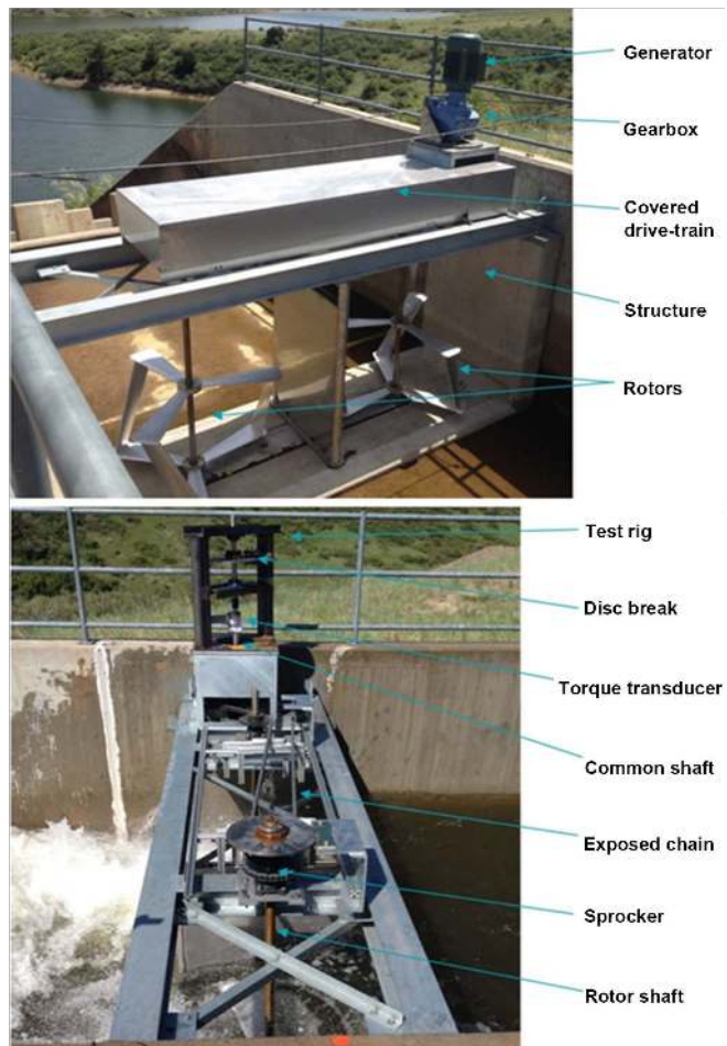
Figure 15. Emrgy's Hydrokinetic Twin Turbine and its main components during testing at Ralston Reservoir. Top, operational set-up including generator, gearbox and drive-train-cover. Bottom, test set-up including disc break, torque transducer/encoder and exposed chain drive.
