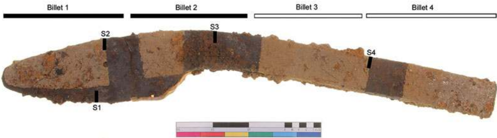
Figure 7. Locations of metallographic sections and the iron billets used in the construction of the couler; billets 1–2, marked in solid boxes, are based upon visible weld-lines, whereas billets 3–4 (open boxes) are inferred from metallographic analysis.
