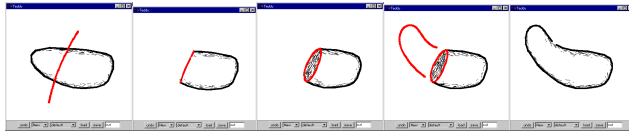
a) cutting stroke b) result c) rotated d) extruding stroke e) result
