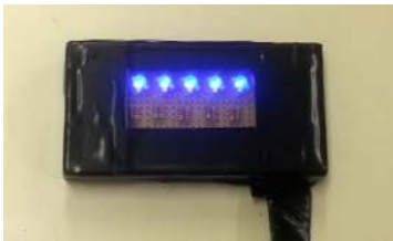
Fig. 2. Screenshot of the RGB LEDs based module. RGB LEDs are positioned so as for their relative positions to be similar to those of the human fingers. The RGB LEDs from left to right correspond to the following fingers; thumb, index, middle, ring and pinky. Such a positioning helps the user to more easily associate the RGB LEDs with the corresponding fingers.
