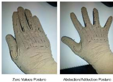
Fig. 6. The two postures used by the calibration procedure. The zero values posture and the maximum abduction/adduction posture.
