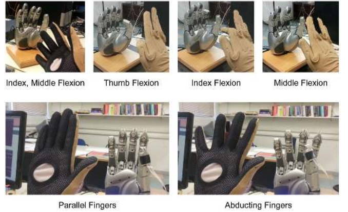
Fig. 7. Different postures of the human and robot hands, representing the different instances of the teleoperation tasks. The Cyberglove II motion capture system was used to teleoperate the DLR/HIT II robot hand in different postures, performing different motions with various speeds.
