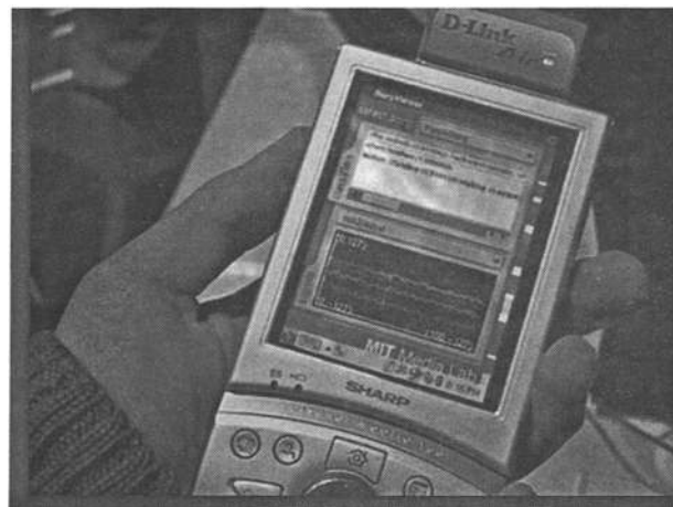
Figure 5. MIThril LiveNet wearable performing real-time analysis and activity classification on accelerometer data and visualizing the results, as well as wirelessly streaming real-time EKG/GSR/temperature and classification results to a remote computer with a projection display, as well as to peer LiveNet systems that may be anywhere in the world. From "Wearable Feedback Systems for Rehabilitation," by M. Sung, C. Marci, and A. Pentland, 2005, Journal of NeuroEngineering & Rehabilitation , 2, p. 17. Copyright 2005 by Sung et al.; licensee BioMed Central Ltd. Reprinted with permission.
