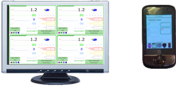
Fig. 1. Patient PDA (right) and Central Station (left) of the Visensia telemetry system.
