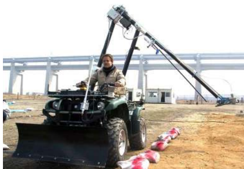
Fig. 3. Gryphon mobile platform can be either manually driven and teleoperated. It can server as a commuting vehicle for the human worker.
