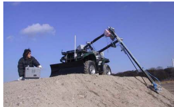
Fig. 6. Gryphon-IV demonstrating the manipulator long-reach capability and the possible application for scanning operation in steep slopes.
