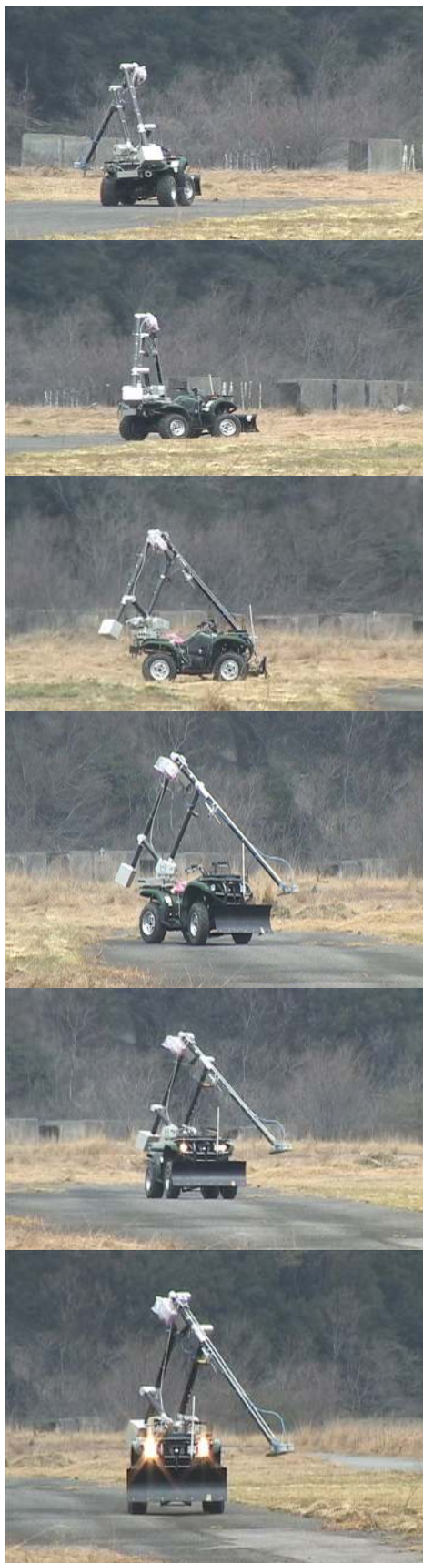
Fig.10. Gryphon-IV remote maneuvering experiment. The system can be remote-controlled in a range of about 150meters.
