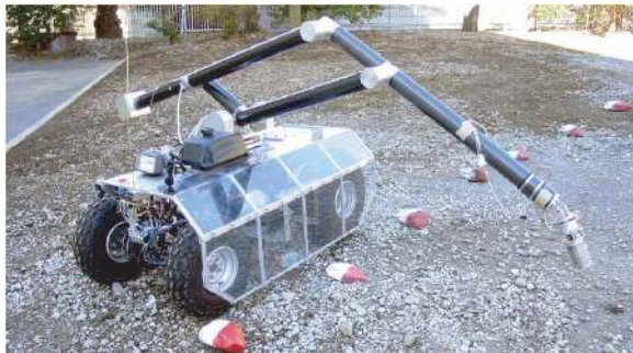
Fig. 7. Former model Gryphon-III equipped with prodder capable of digging the ground. Note that although this is a smaller buggy than the used in Gryphon-IV, the basic automation functions are the same.
