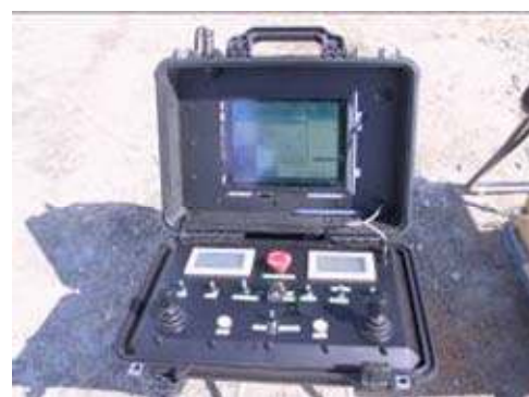
Fig. 4. The remote controller is equipped with two joysticks and few switches. The display panel is in fact a panel computer
