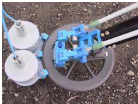
Fig. 8. Sensor head. The left cylinders are the GPR transmitter and receiver antennas, and the right circular sensor is the metal detector CEIA MIL-D1.
